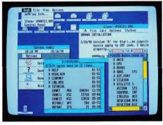
TT's analog RGB 14-inch system outperforms VGA with a multitude of resolutions ranging from 320 x 200 to 640 x 480 with 16 colors
